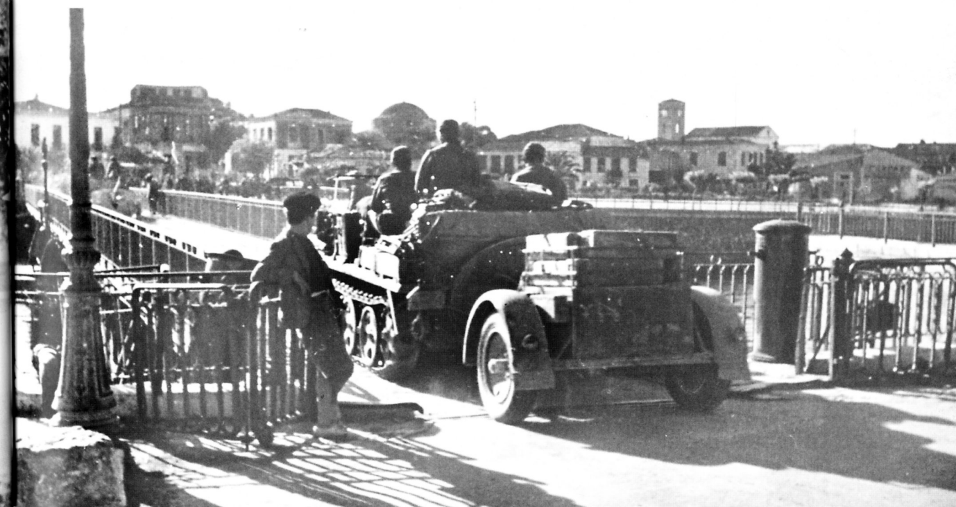
An Sd.Kfz.10 halftrack crosses a bridge in Greece towing an ammunition trailer. The body of the vehicle was entered by climbing over the side, and the interior could be covered from the weather by a fold down canopy and side curtains with clear windows.
