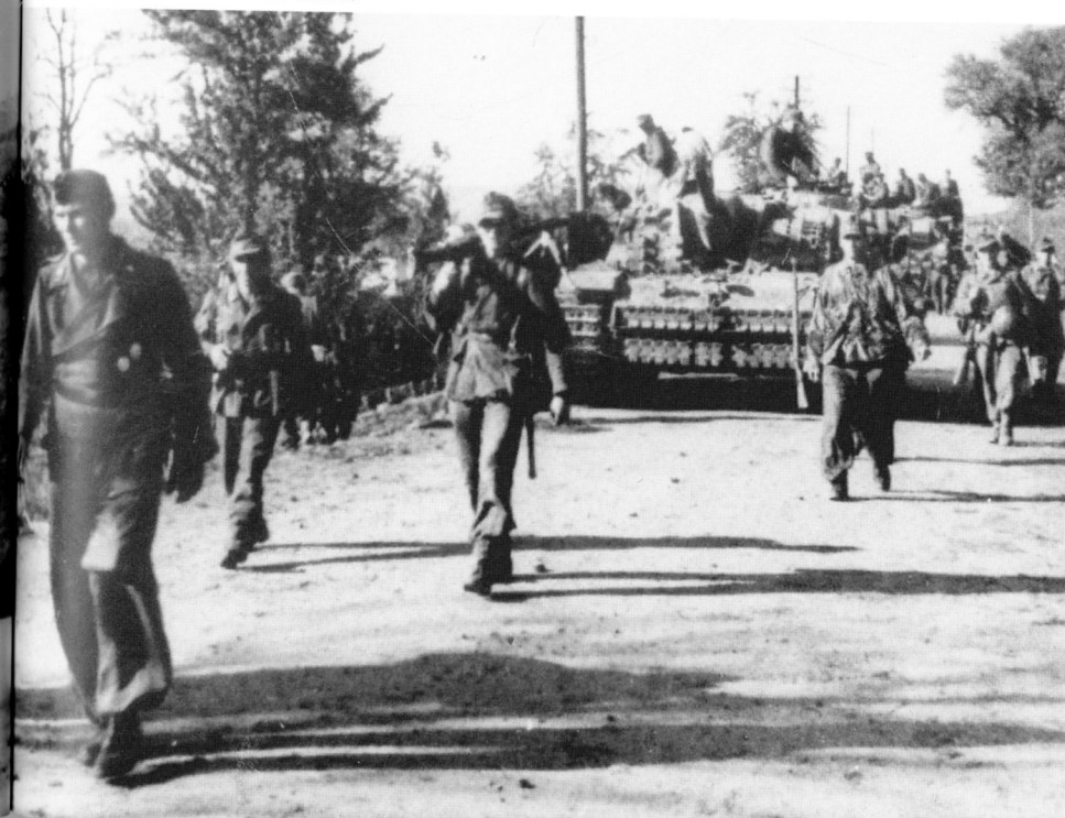
Panzergrenadiers hitch a ride onboard a StuG.III Ausf.G during heavy fighting in the Normandy sector in July 1944. The vehicle still has a protective sleeve over the muzzle break of the barrel. The camouflage scheme over the intact Schürzen is green and brown wavy lines applied over the dark sand base.
