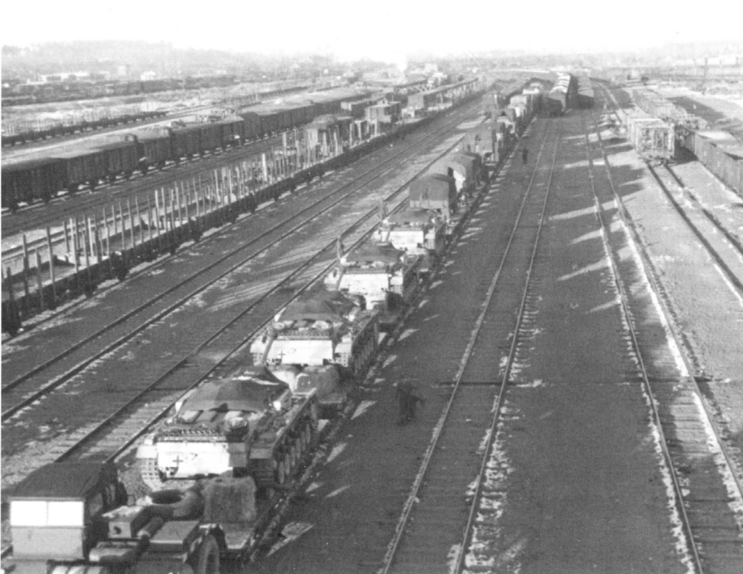
An interesting photograph taken in 1944 showing a long column of StuG.III. Ausf.G's on specially adapted railway flatcars, destined for the frontlines in Russia. Note the lashed down tarpaulins on the vehicles. These were meant to protect sensitive parts of the assault guns from dirt, dust and moisture.
