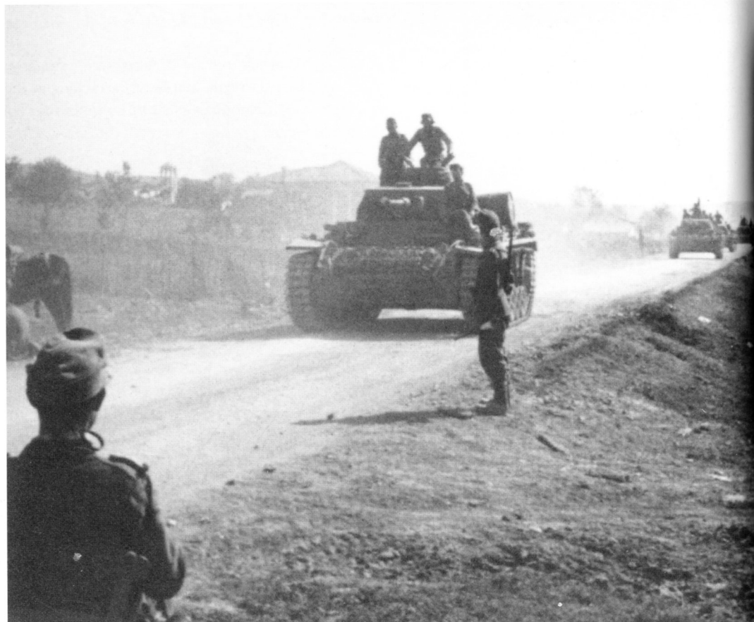
A Pz.Kpfw.III moves along a road during the early spring of 1942. The vehicle has two sets of track links bolted to the front of its hull for additional armoured protection. As with many vehicles of this period the Panzers were still painted in overall dark grey.
