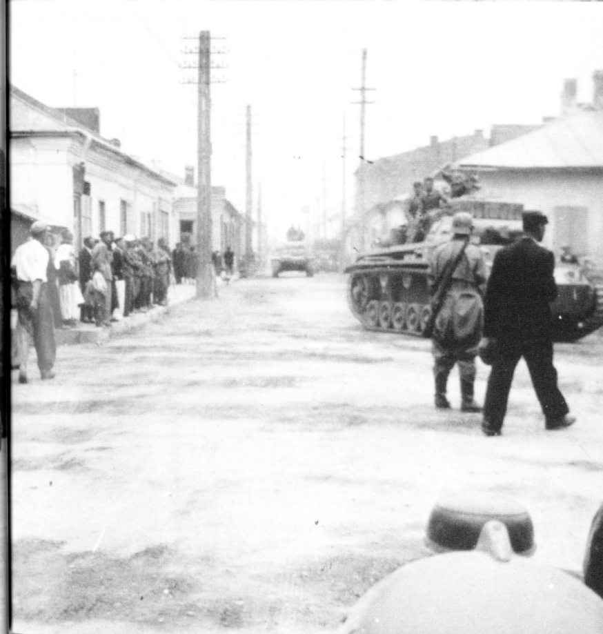
A column of heavily laden Pz.Kpfw.III's from the 46.Panzer-Korps during its furious drive on Belgrade in early April 1941. The crew have stowed a number of items over the engine deck, including supplies and rolled-up canvas sheeting. Note the spare wheels attached to the rear for additional armoured protection.
