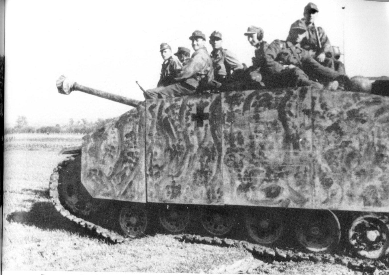
Panzergrenadiers hitch a ride onboard a StuG.III Ausf.G during heavy fighting in the Normandy sector in July 1944. The vehicle still has a protective sleeve over the muzzle break of the barrel. The camouflage scheme over the intact Schürzen is green and brown wavy lines applied over the dark sand base.
