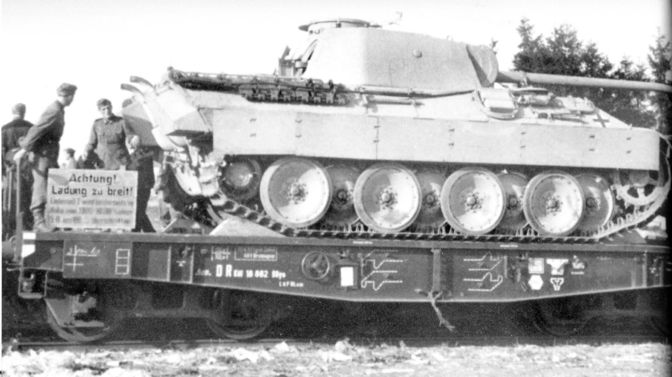
A Pz.Kpfw.V 'Panther' Ausf.D being prepared to be transported from the Italian front to northern France during the summer of 1944. The vehicle still retains its sand base camouflage colour scheme for the Italian campaign, and has no application of Zimmerit anti magnetic mine paste.
