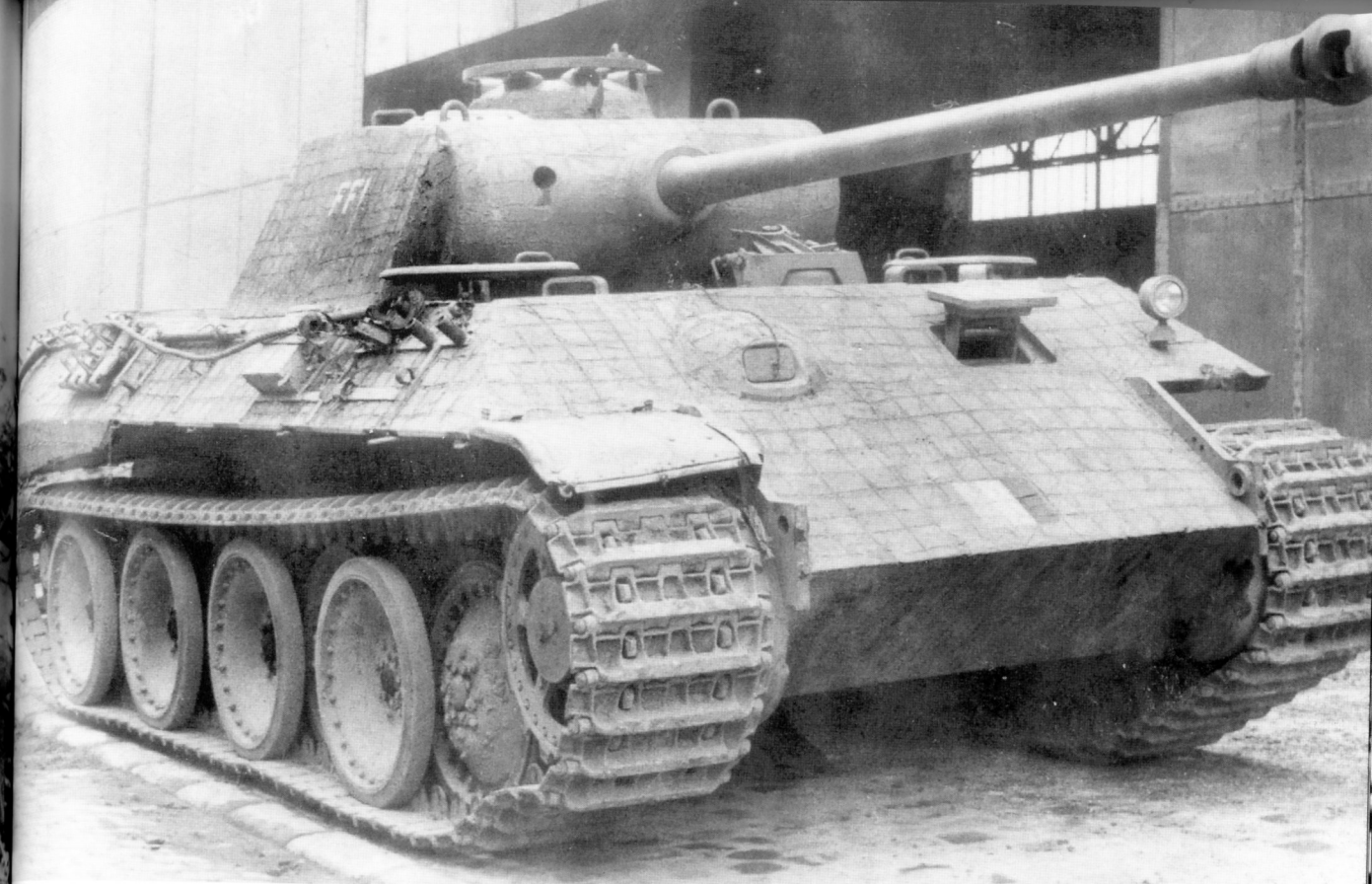
A Pz.Kpfw.V 'Panther' Ausf.D with the preparation of Zimmerit anti-magnetic mine paste which can clearly be seen visible over the entire chassis. Although the Panther dominated the battlefields of the latter half of the war, they were never available in sufficient numbers to alter the course of the battle.
