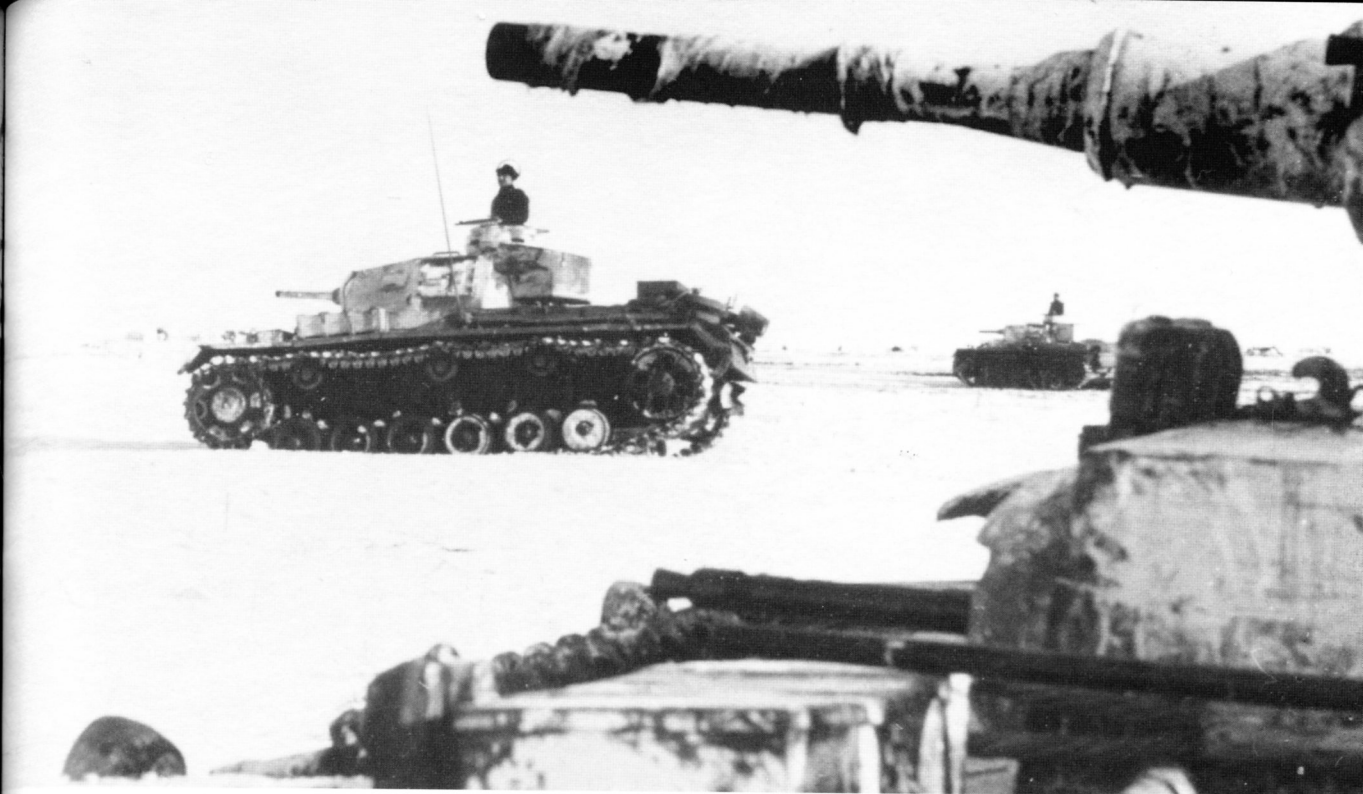
Pz.Kpfw.III's and IV's during the winter battles of late 1942. All of the Panzers have received a very crude coating of winter white wash paint. Once the snow had disappeared crews were able to easily wash off the paint to reveal its original camouflage colours.
