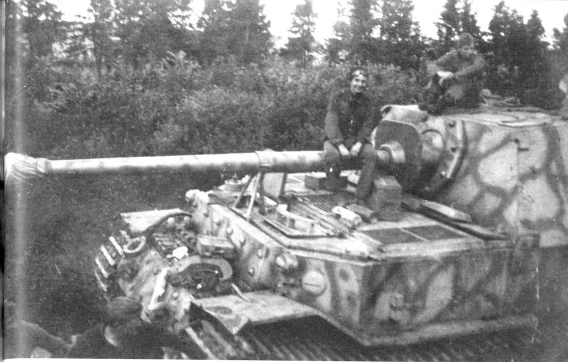
An Elefant tank destroyer stationary on a road with its crew during operations in the later stages of the war. This vehicle saw its debut at Kursk in July 1943 and was able to defeat all types of Soviet tanks, but they lacked cross-country mobility and were prone to breakdowns. Also, with no secondary armament they were vulnerable to infantry armed with magnetic mines and charges.
