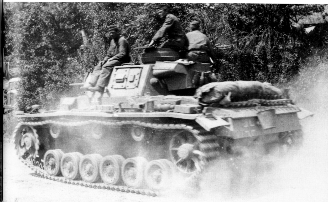
A Pz.Kpfw.III moves along a road churning up dust. Note the rolled-up canvas sheeting on the rear of the engine deck which, when pulled over the top of the vehicle and tied down, formed a kind of canopy and broke up outlines of the tank. The canopy was primarily used to protect the crew from aerial attack by disguising it.
