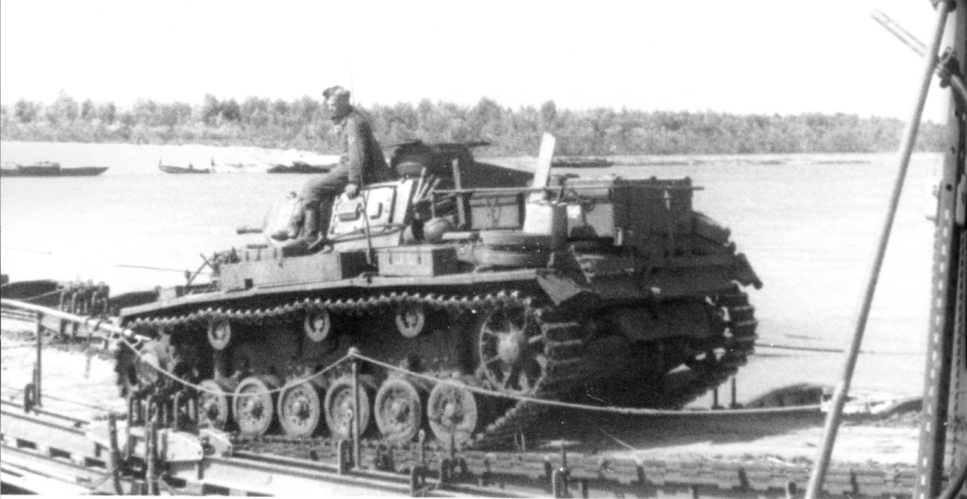
A Pz.Bef.Wg.III command tank crossing a pontoon bridge during operations in the early summer of 1943. Note the prominent rod antenna mounted on the left side and the frame antenna seen fitted on the engine deck. Inside the frame antenna is a stowage bin.
