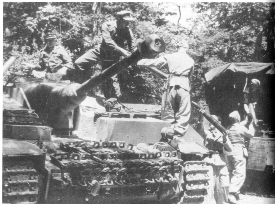
A Pz.Kpfw.IV passes a stationary Pz.Kpfw.VI Tiger.I. Both vehicles have plenty of foliage attached to the turret in order to minimise the high possibility of attack during the daylight hours. Note the attachment of spare road wheels to the rear of the Pz.Kpfw.IV for additional armoured protection.
