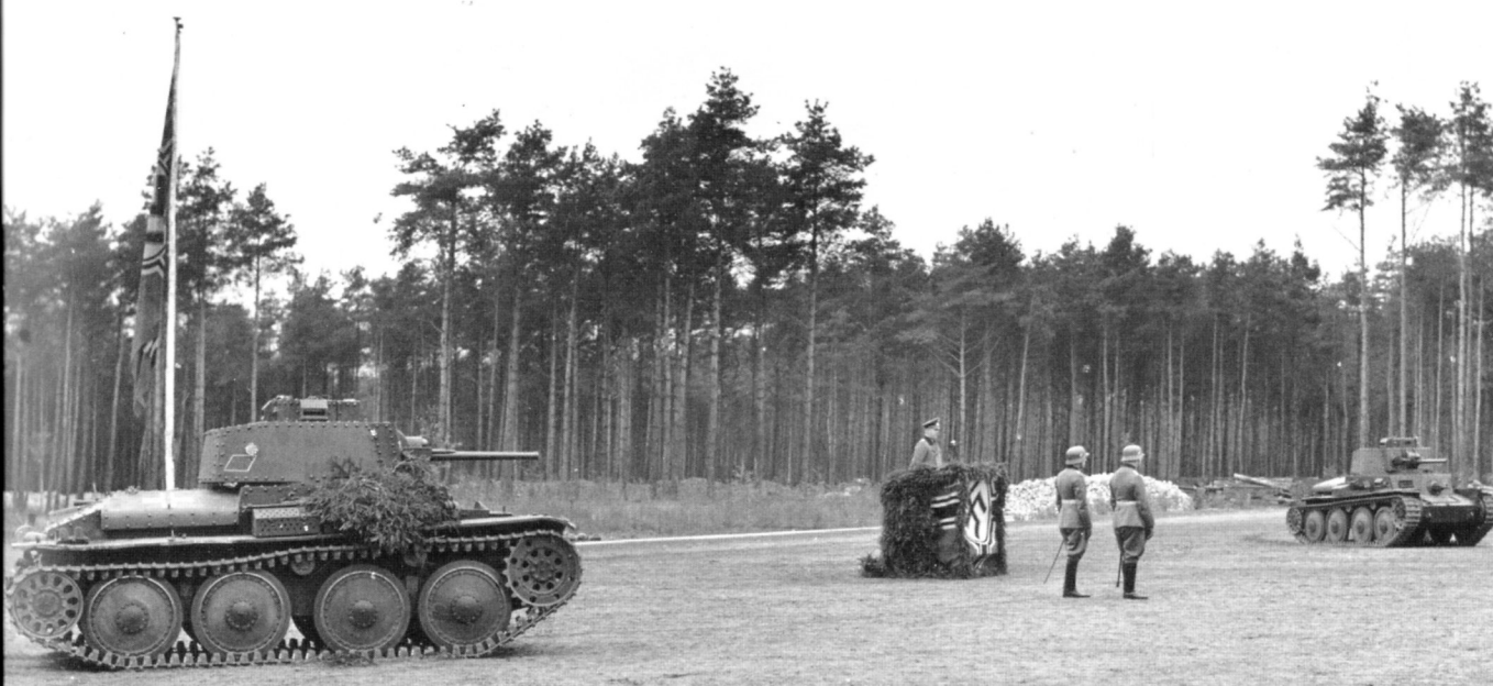
Another military ceremony at a training barracks in 1939. Flanking the commanding officer standing on his podium, are two Pz.Kpfw.38(t)'s. These Czech designed armoured vehicles became the most important tanks used by the Panzerwaffe in the early years of the war. It weighed 9.4 tons. Its main armament was a 3.7cm KwK 38 (t) L/47.8 gun and had two 7.92mm MG37 (t) guns for local defence. Approximately 1400 of them entered service and saw extensive action in the Panzer divisions during the early years of the war.
