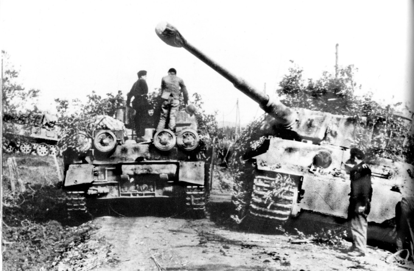
A Pz.Kpfw.IV passes a stationary Pz.Kpfw.VI Tiger.I. Both vehicles have plenty of foliage attached to the turret in order to minimise the high possibility of attack during the daylight hours. Note the attachment of spare road wheels to the rear of the Pz.Kpfw.IV for additional armoured protection.
