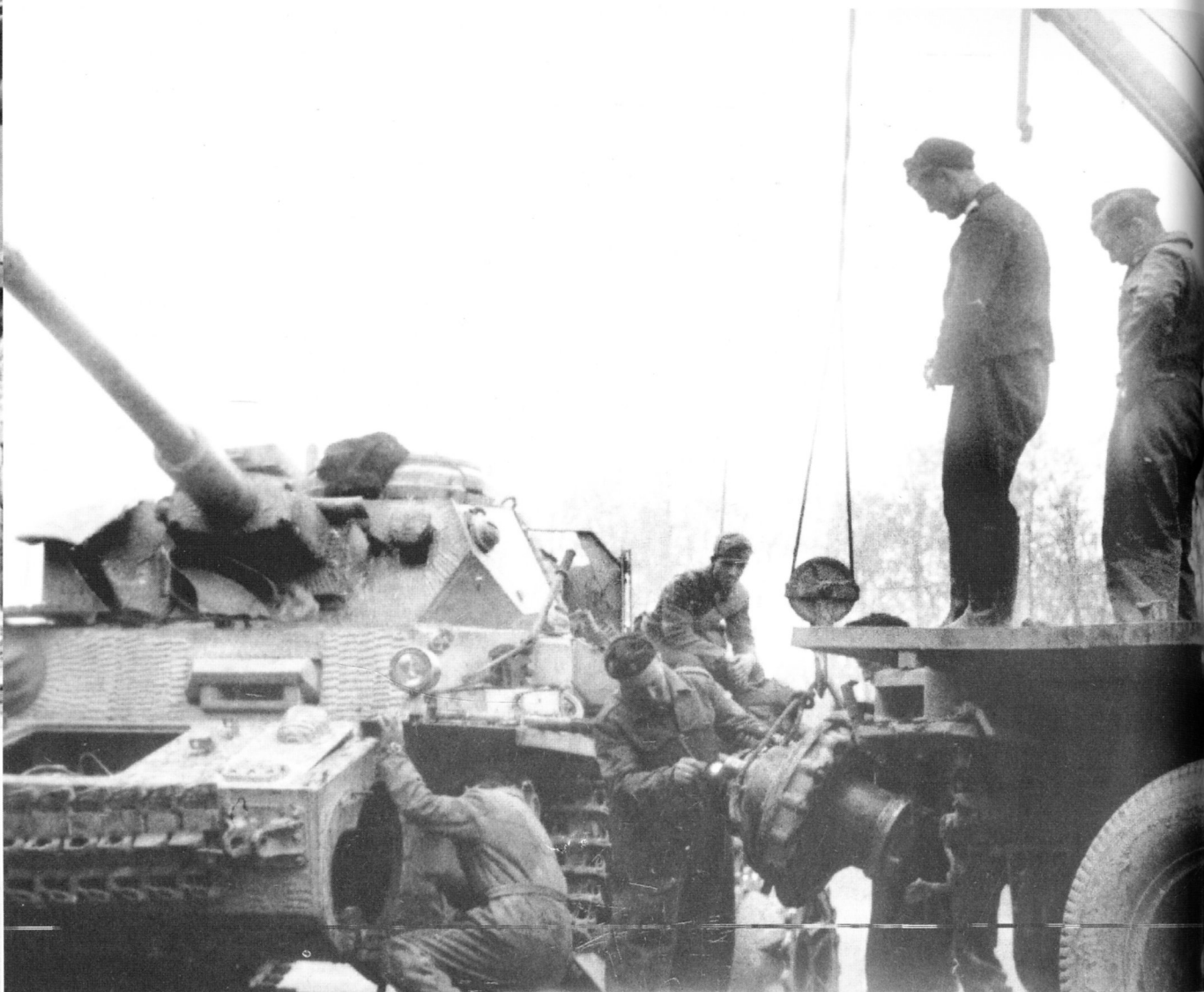
Undertaking repairs to a Pz.Kpfw.IV in 1943. Much was owed to these maintenance companies, which kept the vehicles in fighting condition. The Panzer is covered with Zimmerit, an anti-magnetic mine coating which began to be applied in the factory to virtually all German tanks and assault guns by September 1943.
