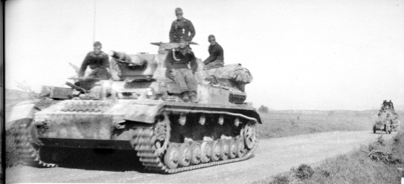
A Pz.Kpfw.IV Ausf.F1 passes along a typical Russian road in June 1941. The Ausf.F1 variant was the first up-armoured vehicle developed in response to heavy allied tanks during the Western Campaign. It was armed with a 7.5cm KwK 37 L/24 short-barrelled gun and was more than capable of dealing with Soviet KV-I and T-34 tanks at short ranges. But by the time the Germans invaded Russia, there were only 548 Pz.Kpfw.IV Ausf.F1's distributed among the Panzer divisions.
