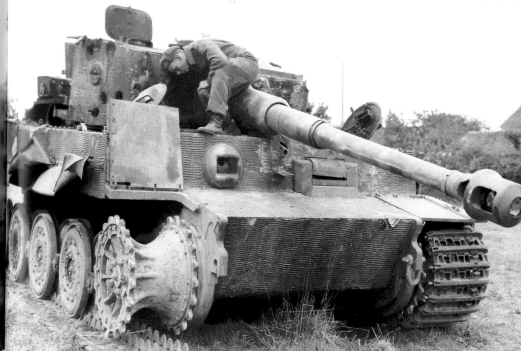
A British soldier examines a knocked out Tiger tank in April 1945. The Tiger has clearly been hit at the side, as twisted skirting is evident from the shells' impact. The loss of the tank track obviously immobilized the vehicle, prompting the crew to bail out. It is unknown whether the crew cannibalised the Tiger first and removed the MG 34 machine gun.
