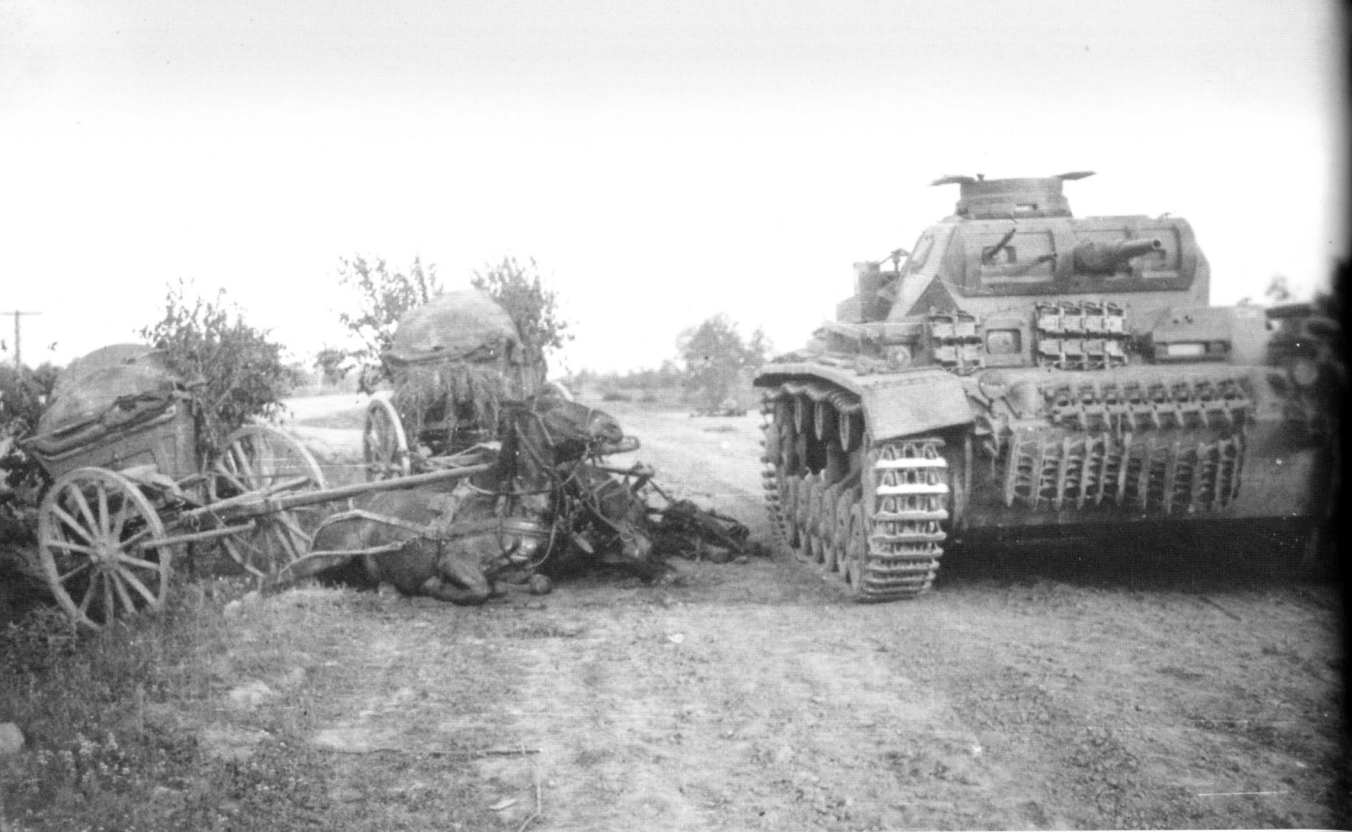
A Pz.Kpfw.III moves along a road during the early spring of 1942. The vehicle has two sets of track links bolted to the front of its hull for additional armoured protection. As with many vehicles of this period the Panzers were still painted in overall dark grey.
