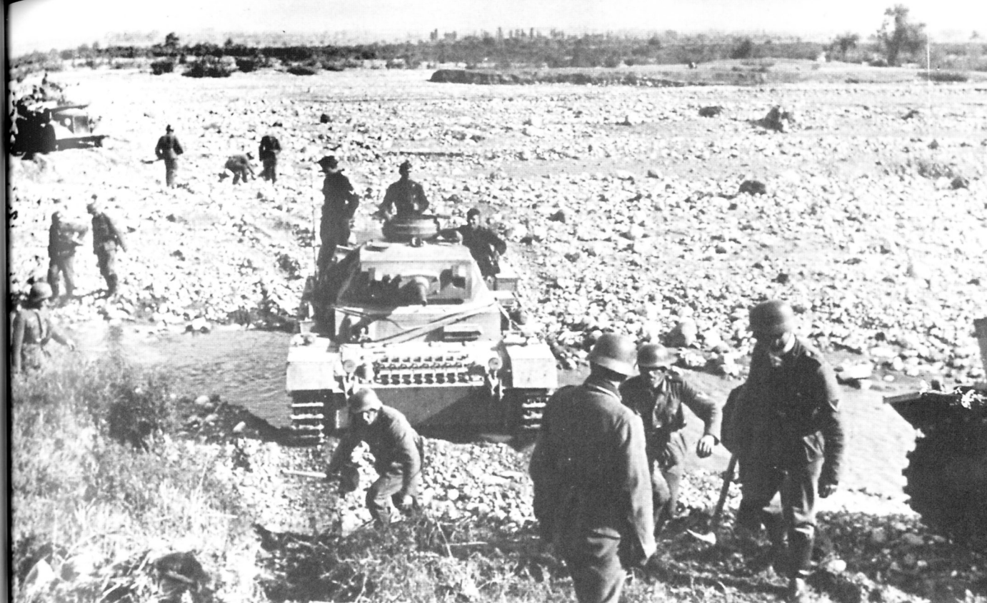
A Pz.Kpfw.III Ausf.G/H moves across some rocky terrain, and following behind is a light Horch cross-country car. Note the soldiers with their short-handled folding entrenching tools. It appears that a number of vehicles have experienced some problems negotiating the uneven terrain, and the drivers have required the soldiers to move some of the larger obstacles out of the way.
