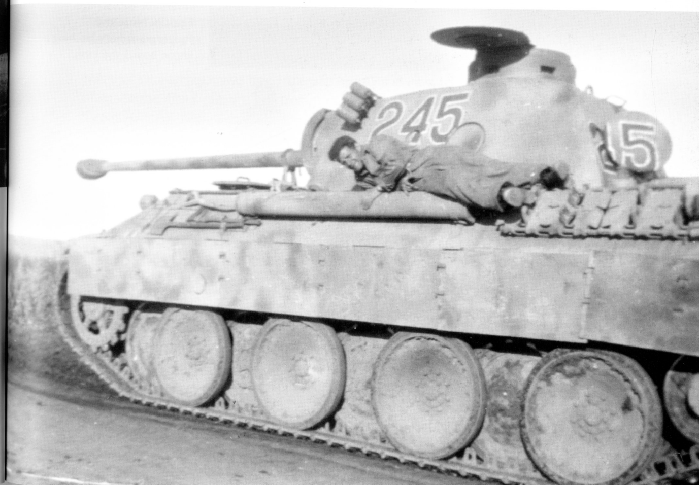
A Pz.Kpfw.V Panther Ausf.D in the summer of 1943. One of the crew poses for the camera sprawled out across the vehicle's gun cleaning tube. The Panther still retains its old smoke candle dischargers that were fitted on either side of the turret. This practice ceased in June 1943 after a reported incident earlier that year, when enemy small arms had set off the dischargers, incapacitating the crew.
