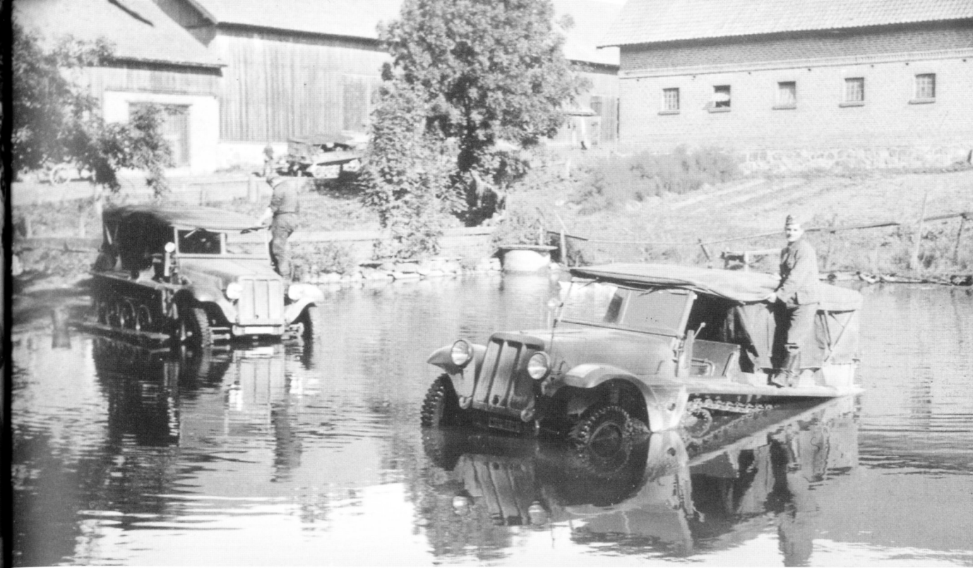
Although a versatile armoured vehicle across varied terrain, halftracks were persistently prone to mechanical problems. They were also liable to develop engine faults in water as this photograph vividly illustrates. It is more than likely that the driver has flooded the engine compartment and is unable to restart the engine.
